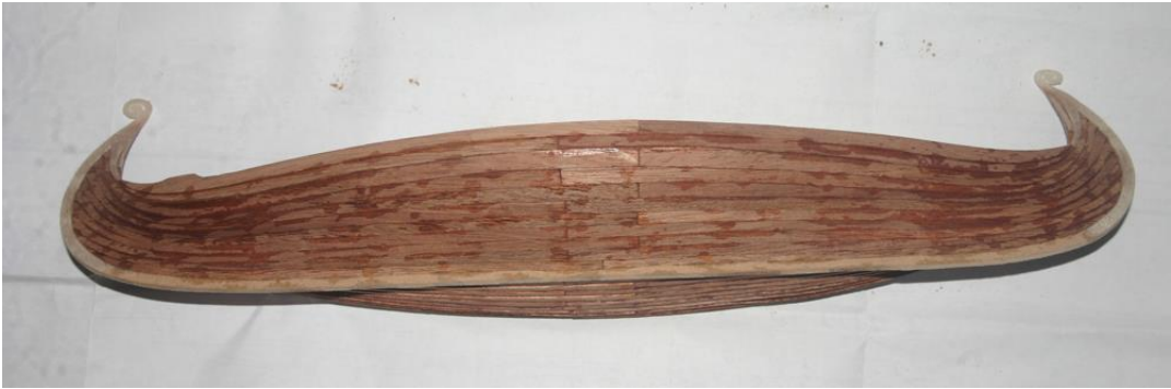
Step 10: Installing buttocks No. 23 & No. 24 at both sides.
